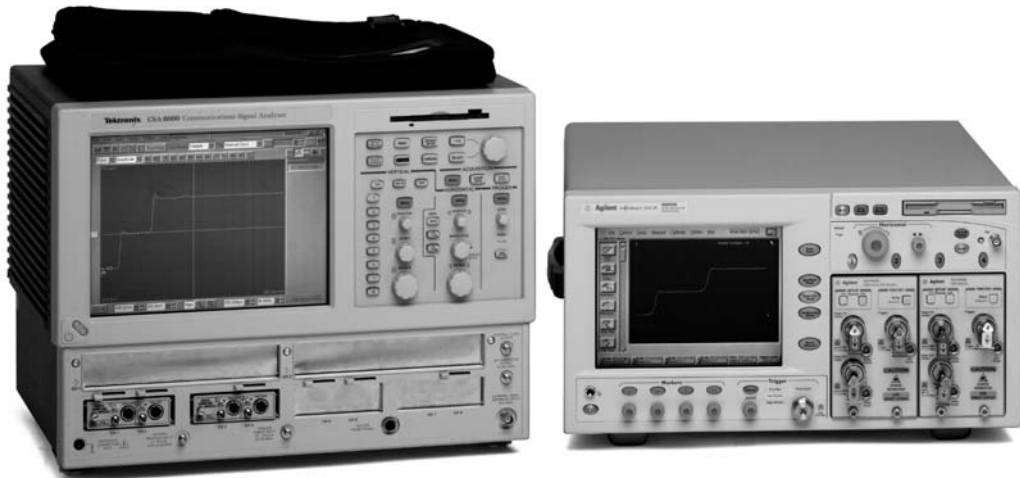
Figure 2-1 TDR-based Physical Layer Test System Hardware: Tektronix CSA8000 (left) and Agilent 86100A/B/C DCA (right)
